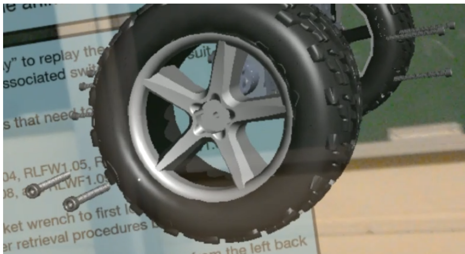
Figure 19: Visualizing the bolt removal process
